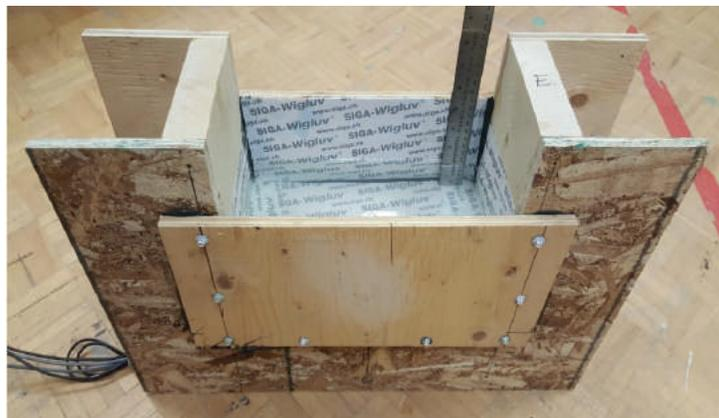
Figure 3 - Typical rough opening frame mock-up lined with Wigluv®
