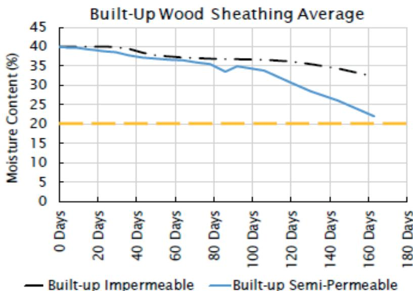
Figure 10 - Built-up sample sheathing moisture content
